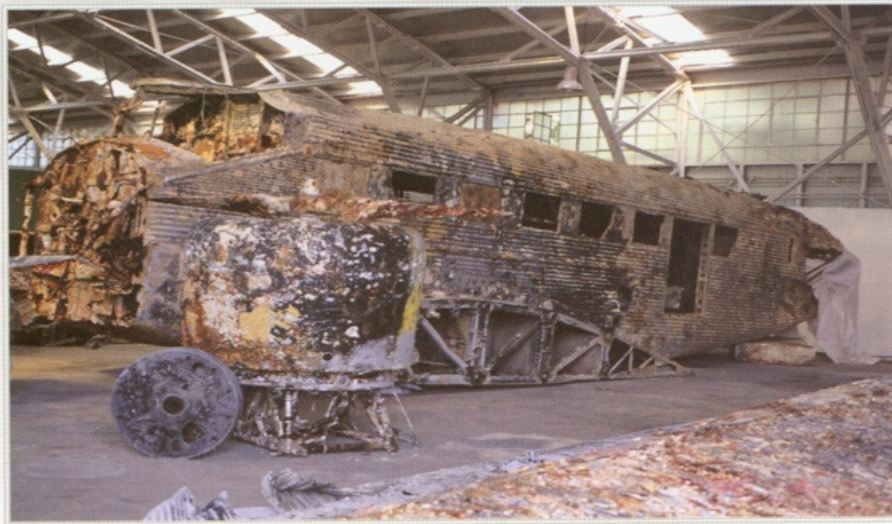
The aeroplane during the final stage of preservation at the Tatoi Air Base. Its wings and engines have been dismantled for transportation.
